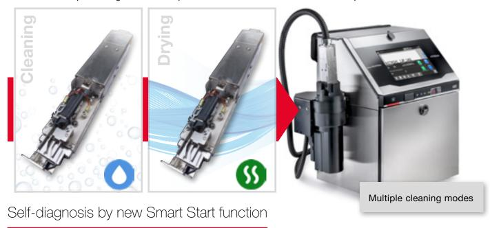
Most of the downtime associated with inkjet printers is a result of a dirty nozzle. The self-diagnosis start-up with Safe clean station can be used to automatically clean the nozzle by reversing the flow of solvent when necessary, which helps ensure that IJP restarts smoothly.
